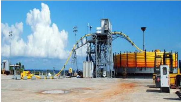
We designed a fully scalable carousel system that can be manufactured to handle 1,000 MT or up to 9,000 MT for the largest carousel, depending on customer requirements. The carousels can be used for land-based storage or offshore deployment of product from an installation vessel.
