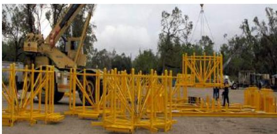
Deep Down's Rapid Deployment Cartridges (RDC) and Subsea Deployment Baskets (SDB) provide installation contractors with safer methods to install umbilicals and flying leads. Both the RDC and SDB provide storage, transportation, and installation methods for your flexible pipe and umbilical flying leads. The RDC and SDB are stackable and typically
