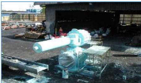
SDV after wet application and all but the flange castings are completed. The flange covers were to be fitted offshore, after installation of the valve.
