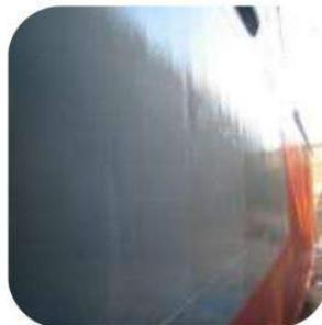
*External surface of a vessel was badly corroded due to the design of the hull. Structural loss was measured at 3-5mm in certain areas. The hull was filled with 100MRP Metal Repair Paste and then over coated with 102 Ceramic Repair Fluid.*
