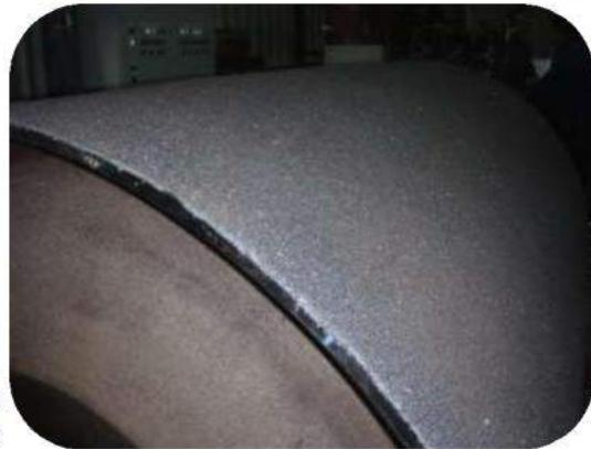
*Conveyor belt roller prepared using needle guns and coated with 100MRF Metal Repair Fluid. Bauxite aggregate was incorporated into the wet resin to create an anti slip finish*
